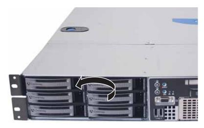
**3** Pull the drive carrier straight out of the server.
